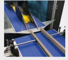
Motorised eletrical adjustable forming inverted head.
