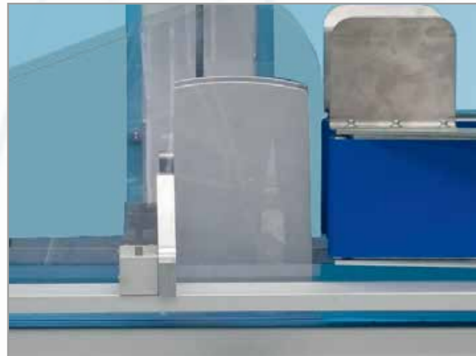
Star rotation system with servo-brushless motor that enables control of the product position during all 90° rotations.
