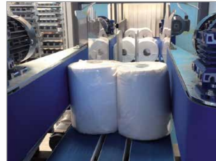
Turns single or multiple products that safely travel between the belts and the automated support conveyor.
