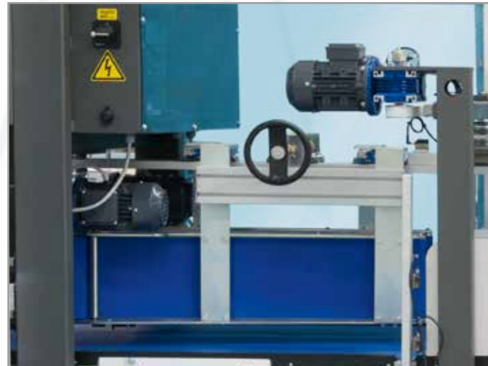
Diverter & launcher to phase the products arriving and to create multiple packs with easy adjustments for simple format change. Composed of automated side belts, for precise exchange of products on channels. Merger for products to transport on a single channel arriving from multiple paths or cutters from multiple channels.
