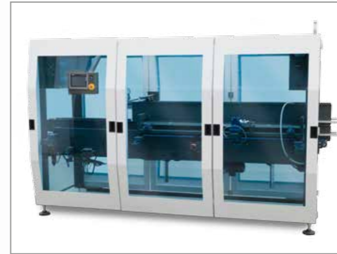
Opening or sliding doors for easy access from both sides.
