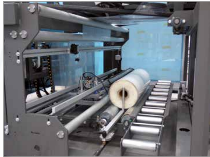
Canter level and accessible from both sides. Reel holder with trolley for easy loading.
