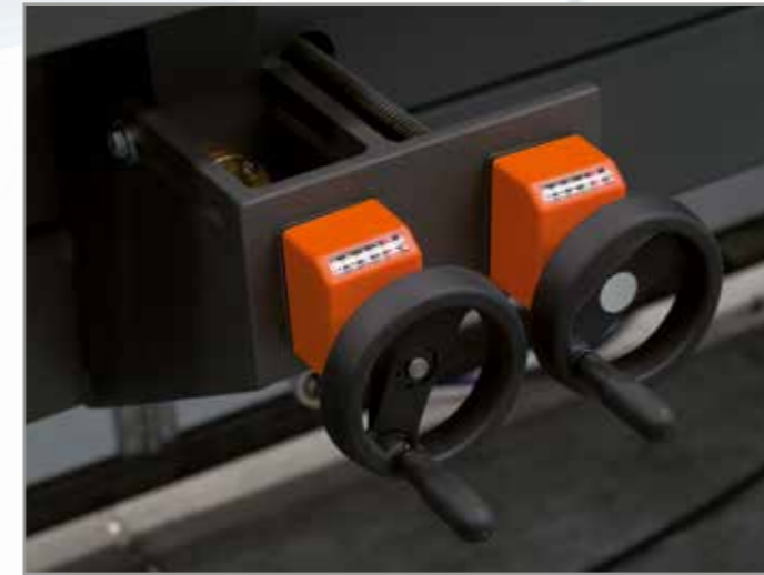
Adjustments for format change, possibly with handwheel with metric rulers or with completely automatic system with motor. Positions can be saved on touch-screen.
