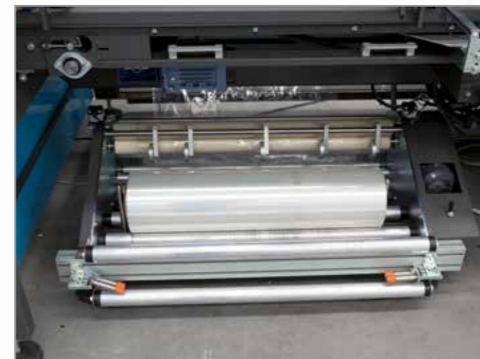
Removable reel holder, for fast reel change. Works with polyolefin and polyethylene film, mono-folding or flat (with external double or single mono-folding machine).
