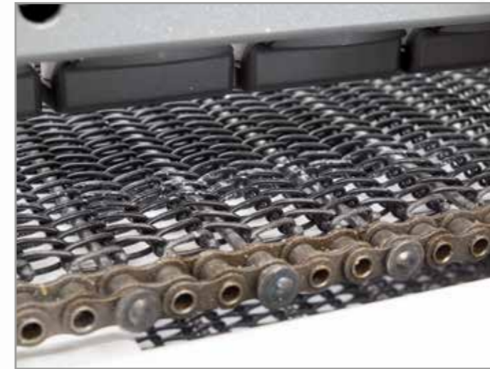
Conveyor belt with Teflon metal mesh or rollers, according to the size of the tunnel and the type of film.
