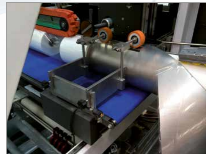
Double sealing device. In the same machine, thanks to the forming tube, you can have: a side sealing system, with overlapping and lap-seal.
