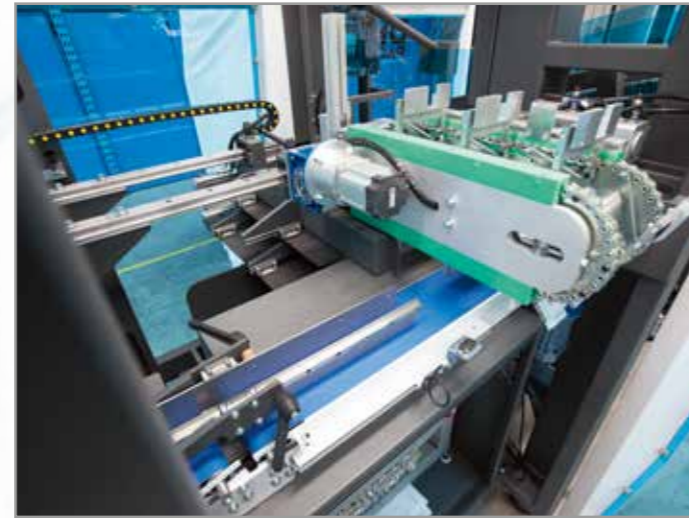
Feeder belt with various types of automatic loading, based on the product.
