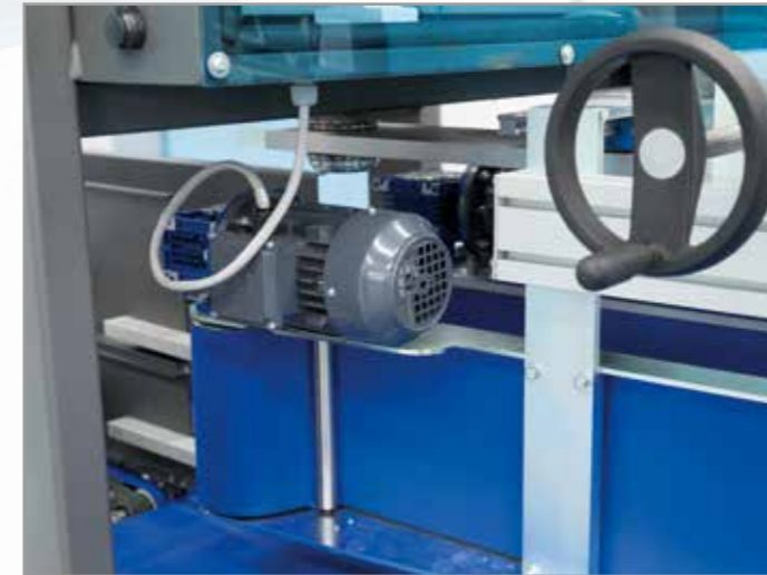
Composed of automated side belts for precise exchange of products and transport on channels.
