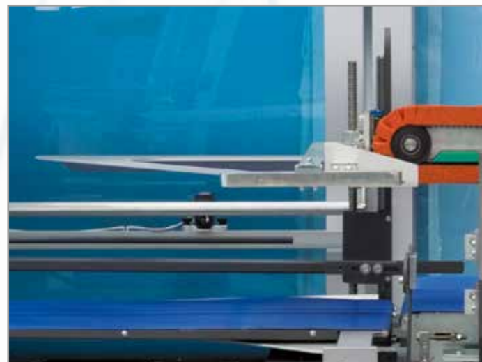
Rounded triangle: enables wrapping the product as a forming tube and saving on film.
