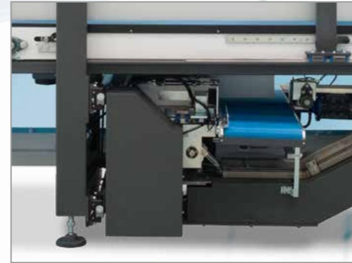
Labels applicator from underneath enabling automatic insertion of the table at high speed between the product and the film, with double automated gripper to guarantee label hold. The applicator is equipped with an automated belt with supports that ensure alignment of the product arriving from the belt above.
