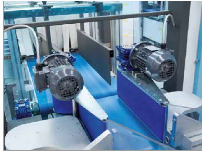
Composed of automated side launching belts to safely send product into the heart of the machine.
