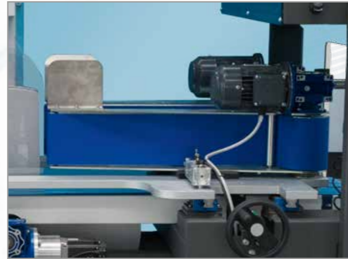
Automated belts also outbound that block and ensure product stability on overturning.
