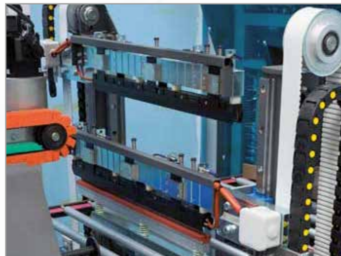
Sealing machine with double bar for high speed. Up to 100 products/min. The double bar ensures the speed and high performance without force for mechanical parts. Available in "lap seal"/top sealing version and overlapping.
