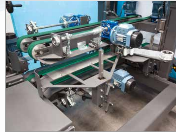
Automatic box closure with adhesive tape or hot glue. Automated side guides. Automatic adjustment.
