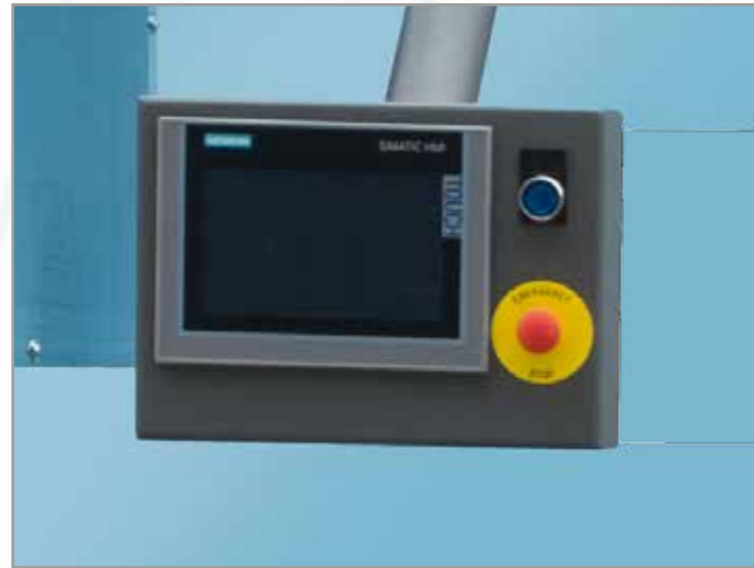
Latest generation touch-screen, can be rotated for machine operation on the right or left.
