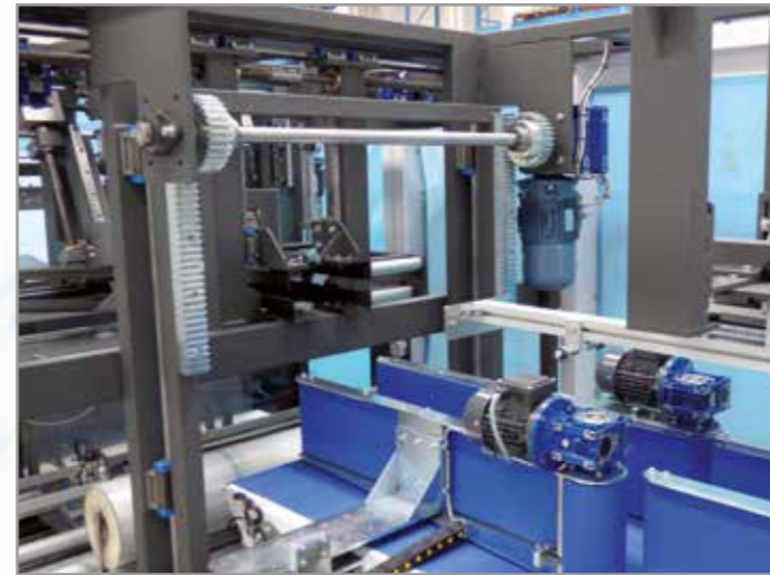
Movements commanded and controlled by servo-motor, to ensure precision, reliability and minimum maintenance. Format change without using tools.
