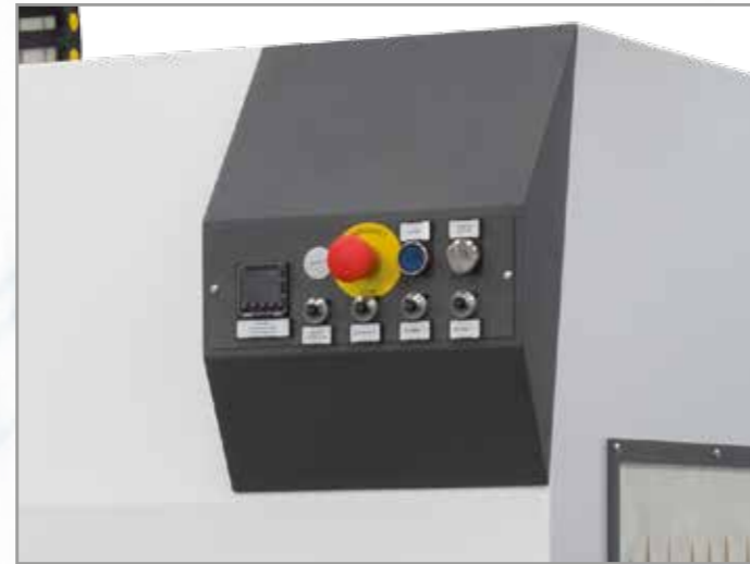
Temperature adjustment with static relays.
