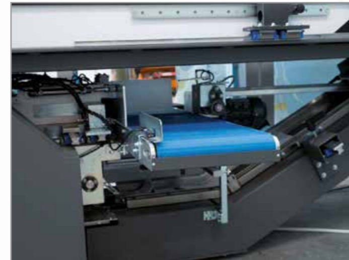
Easily removable thanks to the construction assembled on sliding linear guides.
